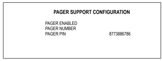
A password is required to enter a pager number and change the pager pin number. See **Figure 48** and **Section 3.2 - Security Access and Passwords.** Press SELECT will return the Operator to the Communications Options Screen. (See **Figure 55**.) To go to the second page of the Communications Options Screen, bracket NEXT and press SELECT. The following screen will come up.
